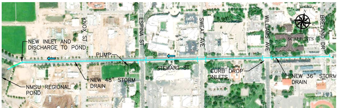
FIGURE 8-5: STEWART ST STORM DRAIN
