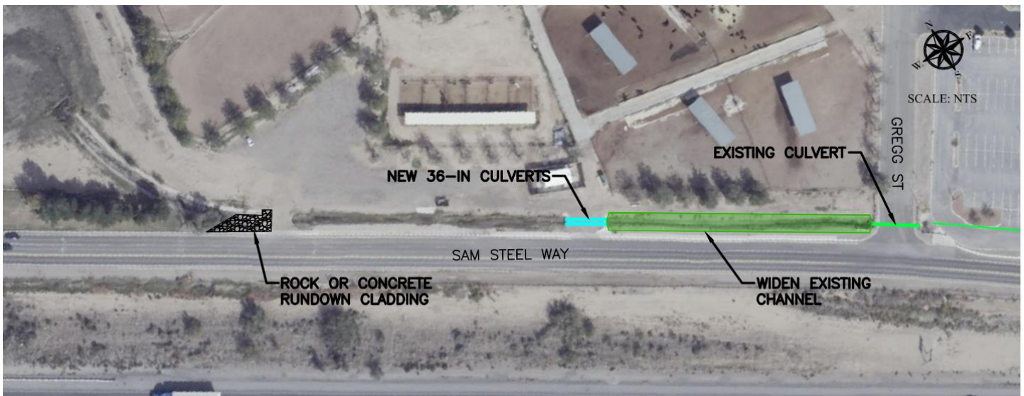
FIGURE 8-13: SAM STEEL WAY IMPROVEMENTS
