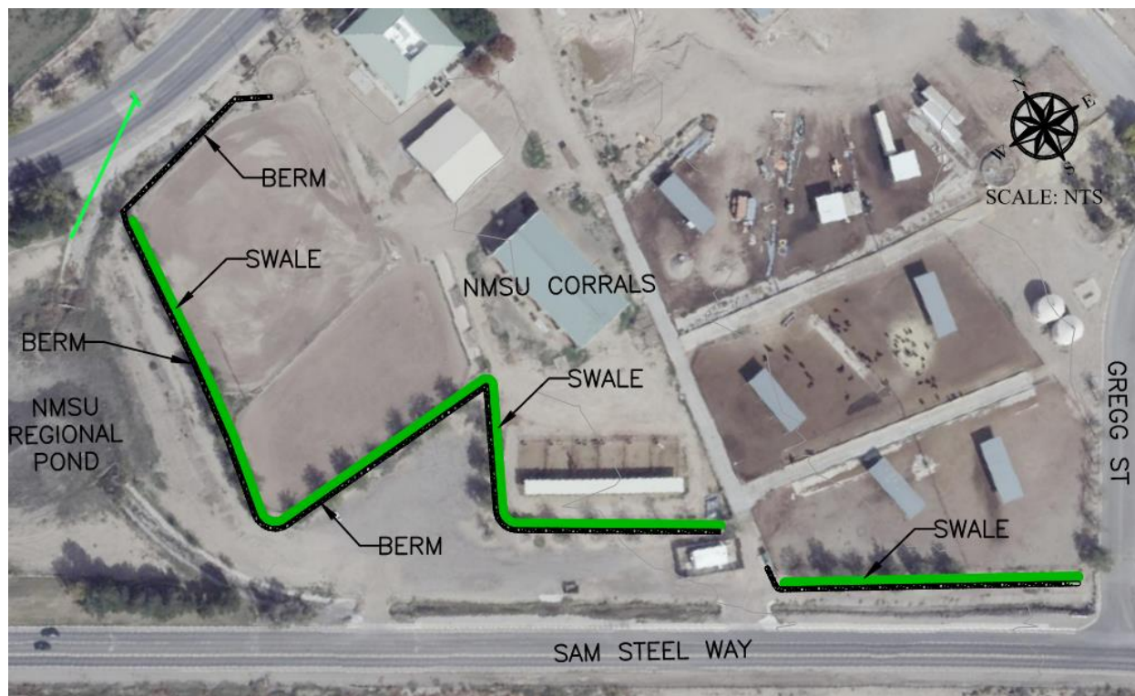
FIGURE 8-15: CORRALS RUNOFF MITIGATION – PLAN
